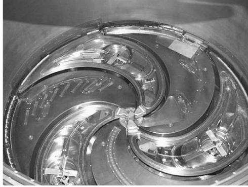
Figure 3.2: View of the cyclotron median plane [50].
