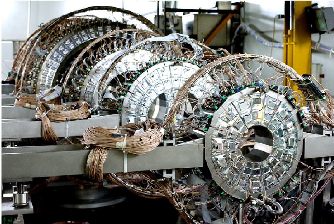
Figure 3.2 Recent photo of the CHIMERA multidetector with sphere and five rings. The other four rings of the forward part have been transferred at GSI.
