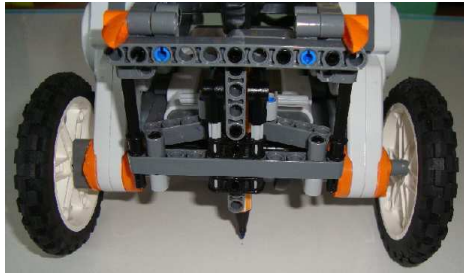
Figure 29 – Robot used for designing the writing robot and the painting robot applications. The paintbrush can be noticed at the center of the axis of the two wheels.
