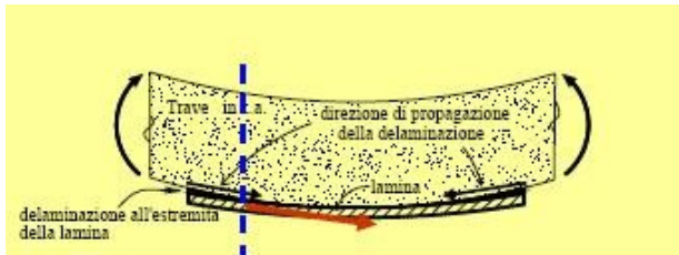
fig 1.j - Failure mode “plate and debonding” debonding”
