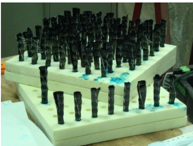
fig. 2.t - The anchor dowels inserted in the polystyrene mould
