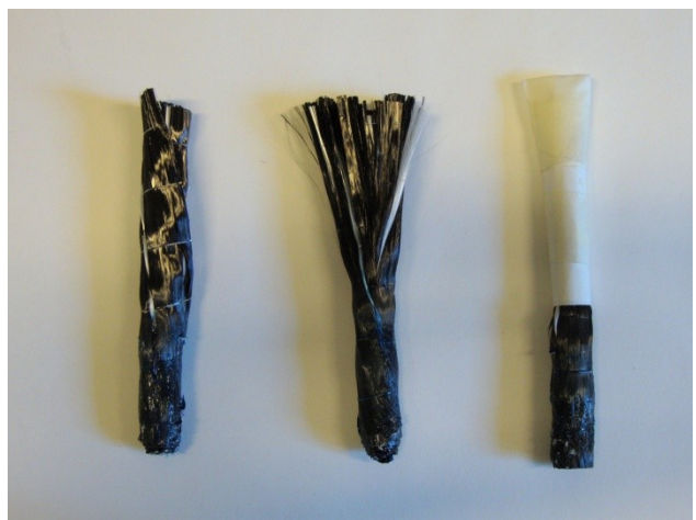
fig. 2.u - The impregnated anchor realized; on the right the anchor ready to be insert in the fire brick
