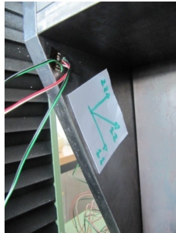
fig. 2.lll - The strain gauge rosettes applied on the critical points of the apparatus. In the images are framed on the left the gauges 1 and on the right the gauges 2. Moreover the name of the axis is shown From each rosette it has been obtained the value e_x , e_y and e_{xy} . To obtain the strains the follows equations have been used.
