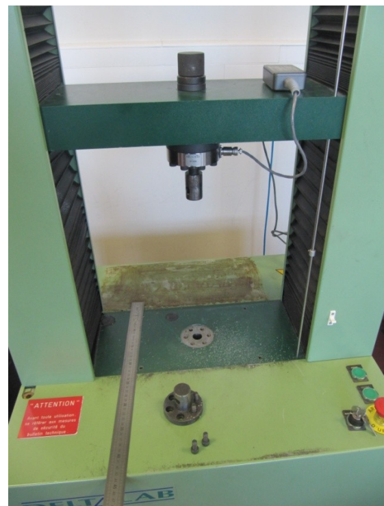
fig. 2.ii - Detail of the universal machine (load cell and bolts joints)
