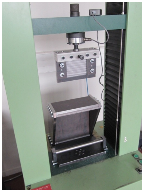
fig. 2.ttt - The steel apparatus assembled in the universal machine
