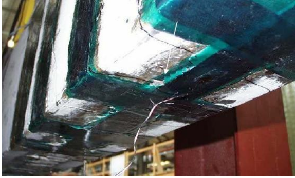
fig. 1.oo- U WRAPS joint system [17]
