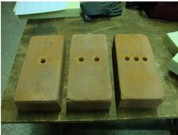
fig. 2.v - The three typologies of support with anchor holes
