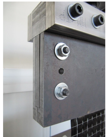
Figures 2.bbbb - The steel grab reassembling and the @ plate clamping; three steps of the procedure
