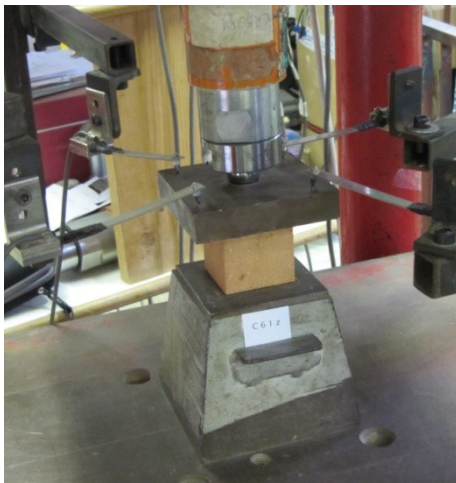
fig. 2.e Compressive test over a cube
