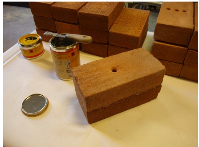
fig. 2.w - The support constituted by two glued bricks
