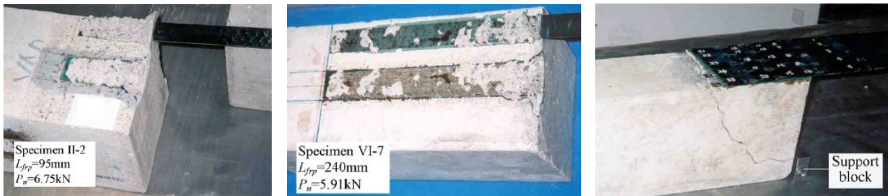
fig. 1.y - Failure modes in the Yao et al. experimental session [6]
