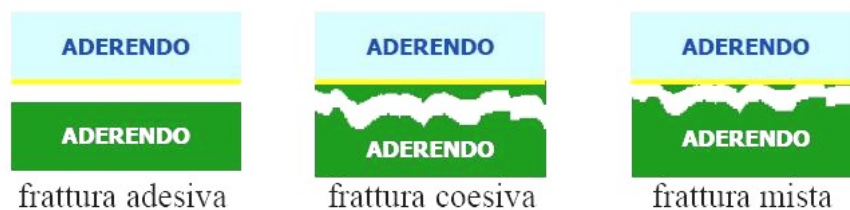
fig 1.i - The main typologies of fracture (adhesive, cohesive, mixed) [1]
