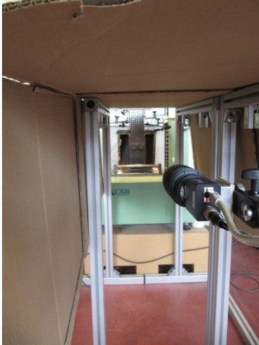
fig. 3.u - The devices used to overshadow the specimen
