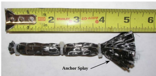
fig 1.ss - Dry fiber anchor [20]
