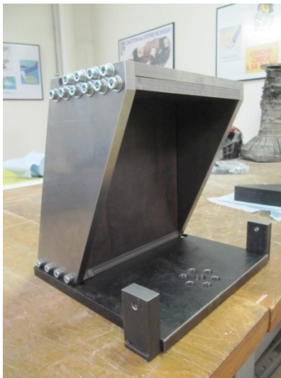
figures 2.jjj - The lateral reinforces of the “Z box”
