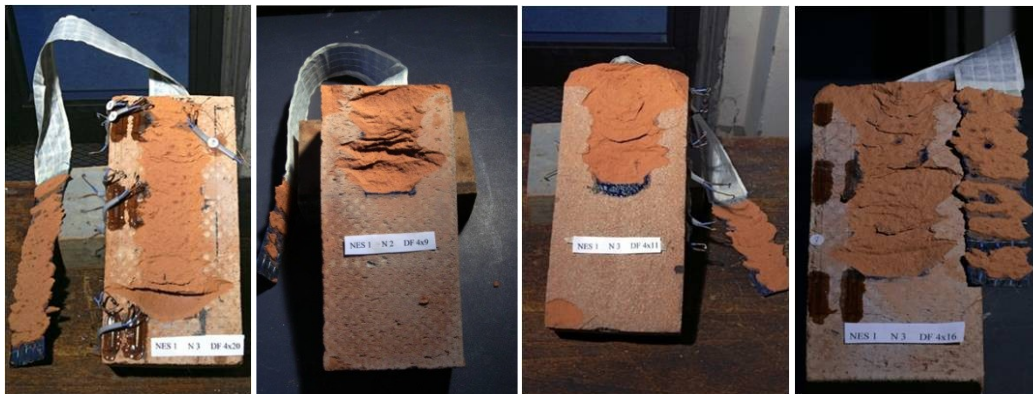
fig. 1.cc - Failure mode, NES double shear tests (a M. Fagone courtesy)
