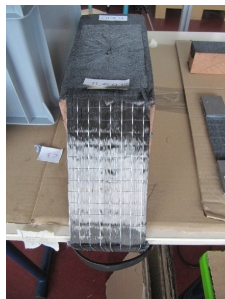
fig. 2.vvv - The device to stretch the fibers and block the plate without touch the adhesive
