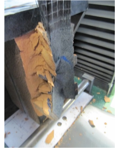
fig. 4.b - The specimen during three test phases; in the left an image of the sample during the crack advancement (strokes BC), in the center a photo of the specimen after the total debonding fracture (strokes DE), finally, in the right a figure of the anchor detached from the CFRP sheet after the achievement of the P_3 .
