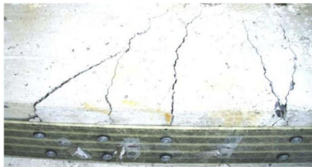
1.nn Crack and nails in a flexural test [15]
