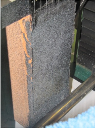
fig. 4.b - The specimen during three test phases; in the left an image of the sample during the crack advancement (strokes BC), in the center a photo of the specimen after the total debonding fracture (strokes DE), finally, in the right a figure of the anchor detached from the CFRP sheet after the achievement of the P_3 .
