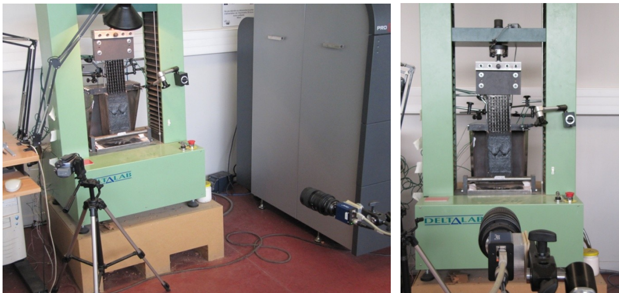
figures 2.ffff - Photo and video camera placement during the tests
