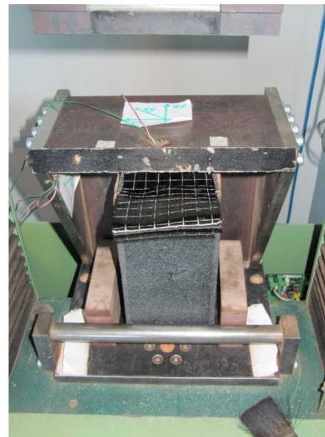
figures 2.yyy - The insertion of the specimen inside the contrast apparatus (photo on the left ) and the reassembling of the Z steel contrast using the two templates 70x140x40)
