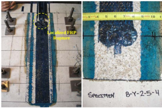
fig. 1.xx - Failure of the specimen with two anchors placed across the width of the sheet
