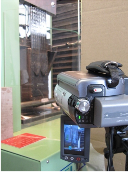
fig. 2.hhhh - The Plexiglas foil interposed between the video camera and the specimen
