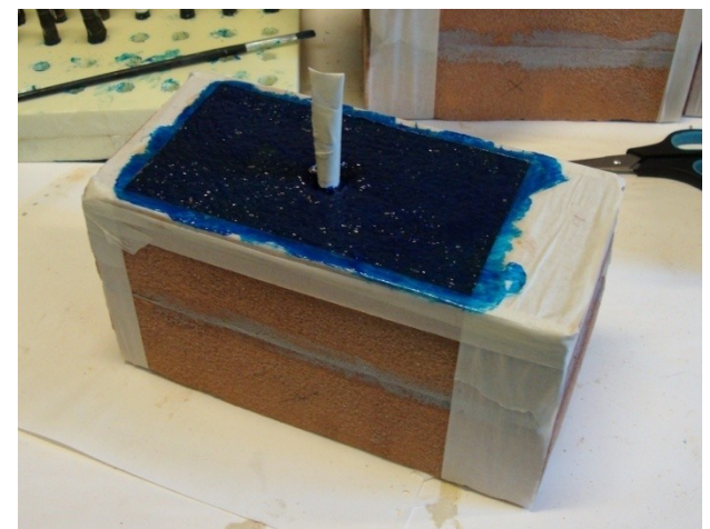
fig. 2.aa - Fire brick surface covered by epoxy resin
