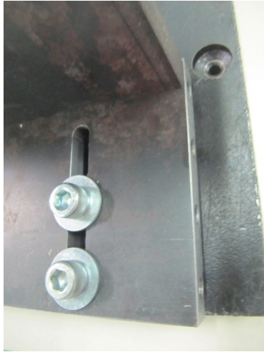
fig. 2.hhh - The bolt joints between the steel support and the Z box.
