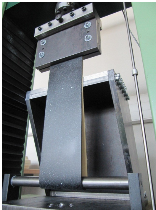
fig. 3.l - The traction test on rubber. Boundary conditions and photos of the test apparatus
