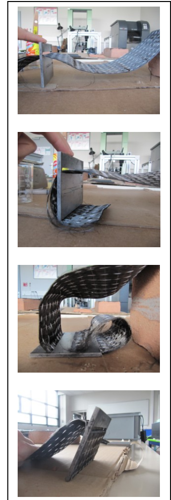
fig. 2.uuu - The fiber carbon to steel plate @ bonded phase; in red the fiber fabric and in blue the adhesive layer. On the right some photos of the procedure.
