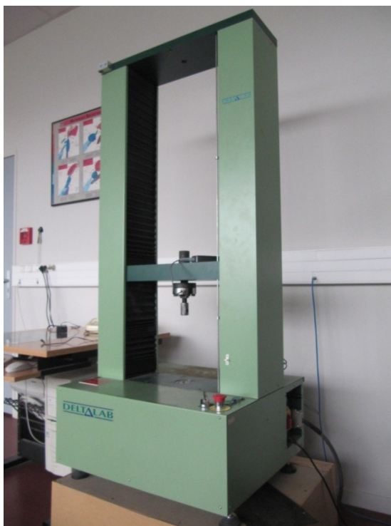
fig. 2.hh - The universal machine EM550 DELTALAB
