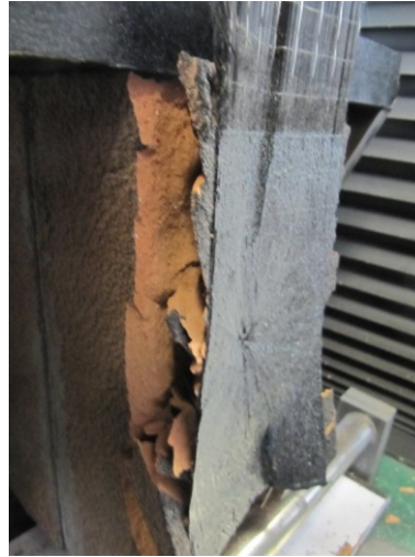
fig. 4.b - The specimen during three test phases; in the left an image of the sample during the crack advancement (strokes BC), in the center a photo of the specimen after the total debonding fracture (strokes DE), finally, in the right a figure of the anchor detached from the CFRP sheet after the achievement of the P_3 .
