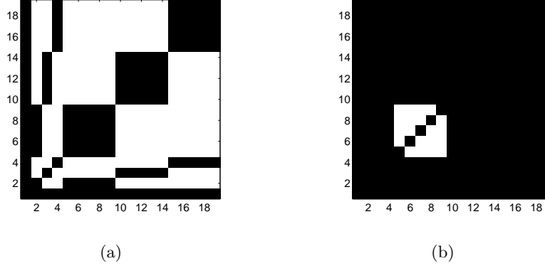
Fig. 5.3. RS links when node 1 (a) or node 2 (b) of the toy model is attacked. The presence of a RS link between i and j is indicated as a white pixel in the i - j matrix. (a) \omega_1 = 2.5 , \omega_i = 1 \pm 5\% \forall i = 2, \dots, 19 , \lambda = 1 ; (b) \omega_2 = 2.5 and \omega_i = 1 \pm 5\% for i = \{1, 3, \dots, 19\} , \lambda = 0.6 .
