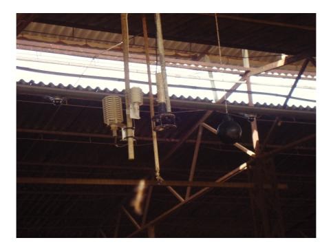
Figure 6.9: Temperature and humidity sensors, anemometers and globe thermometers within the study area.
