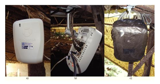
Figure 6.11: Sensors IP30 Serie 7000 used in the trial. a) front side of a sensor; b) back side of Master sensor with 'Timing Cables' (black) and power cable (white); c) sensor covered with protective plastic material.
