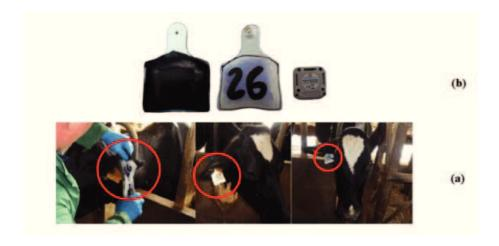
Figure 6.23: (b) Protecting wrapping of tags (front and back) and a Compact Ubisense Tag. (a) Application of the tags to three cows.
