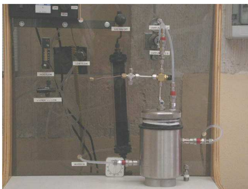
Figure 2.4 - Retronasal Aroma Simulator apparatus (CoRFiLaC Laboratory)
