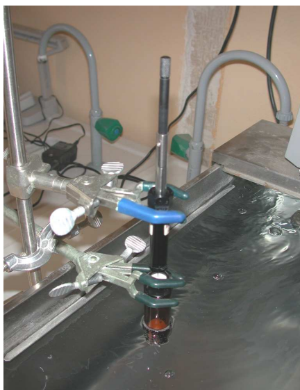
Figure 2.2 - Schematic illustration of SPME sampling (CoRFiLaC Laboratory).
