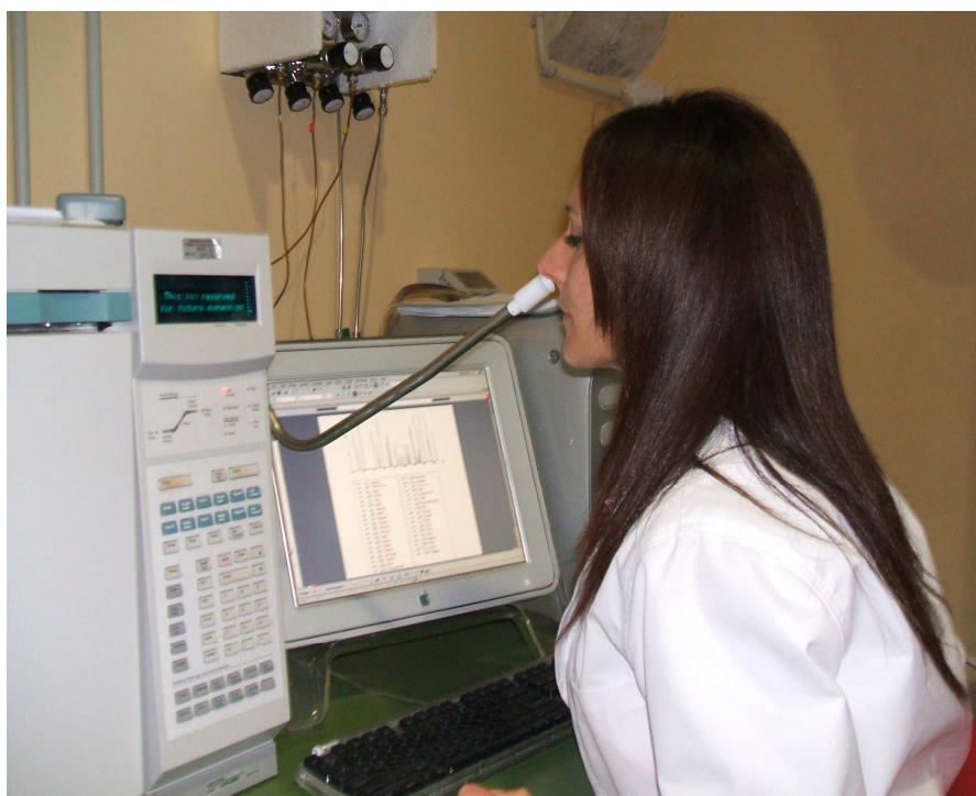
Figure 3.8 – GC-Olfactometer (CoRFiLaC Laboratory).
