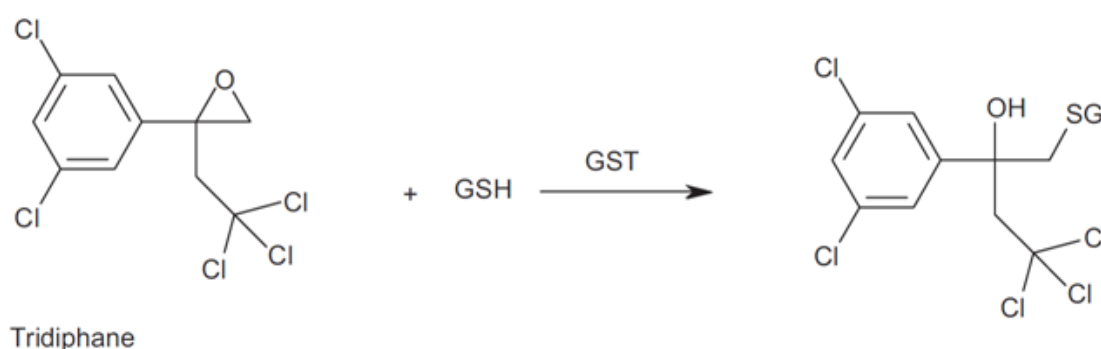
Fig. 1.12 Conjugation reaction of tridiphane to GSH catalysed by GST.
