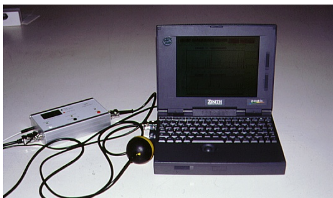
Figure 1.2: Instrumented Sphere PMS 60 developed at ATB.
