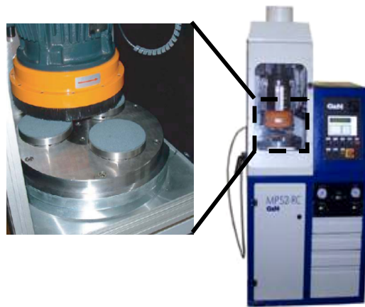
Figure 4.1 Grinding machine G&N MPS2-RC Vacuum.
