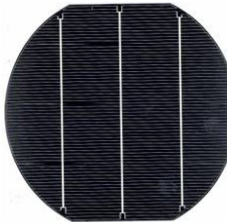
Figure 4.33 Front contact realized by screen-printing process.
