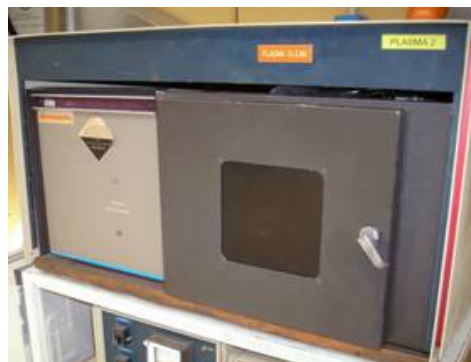
Figure 4.26 Used reactive ion etching equipment.
