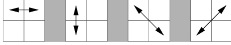
Figure 4.8: Four directions of adjacency as defined for calculation of the Haralick texture features. The Haralick statistics are calculated for co-occurrence matrices generated using each of these directions of adjacency.
