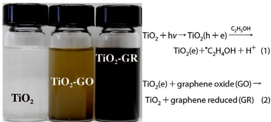
Fig. 1.4.4 – Color change of a 10mM solution of TiO 2 nanoparticles with 0.5 mg/mL GO before and after UV irradiation for 2 h in ethanol. A suspension of 10 mM TiO 2 nanoparticles is also shown for comparison [108].
