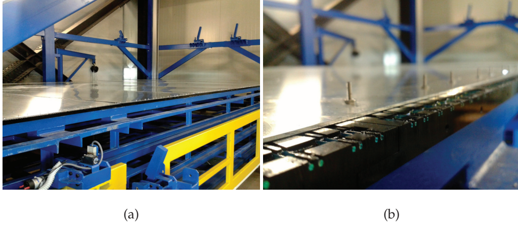
Figure 2.6: Picture of the first logical plane (X-Y) which has been recently assembled and positioned on the mechanical structure (a), particular (b).
