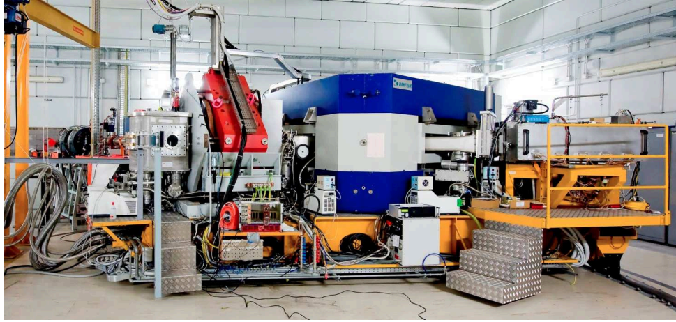
Figure 3.3: General view of MAGNEX spectrometer. From the left to the right the scattering chamber, the quadrupole (red) and the dipole (blue) magnets, and the FPD are visible.
