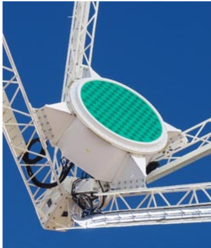
Figure 2.3: Phased Array Feed mounted on an ASKAP antenna.
