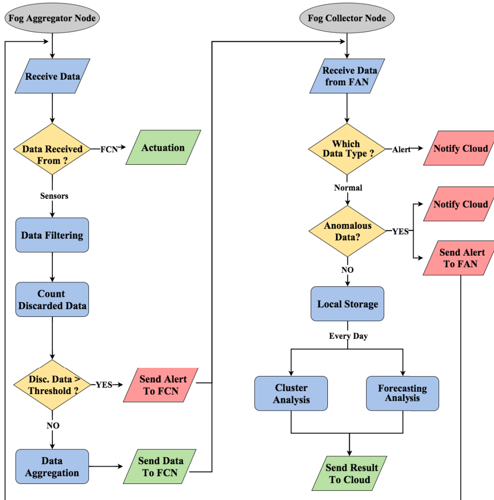
Figure 11 - Flow diagram which describes the Fog logic
