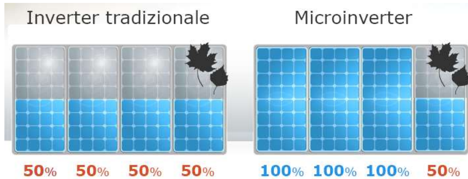
Fig 3.27-a – Micro-inverter advantages against shadowing.
