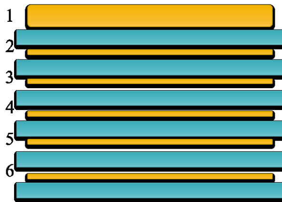
Figure 6:79 Schematics of the composite laminate prepared with OPTESat electrospun nanofibers
