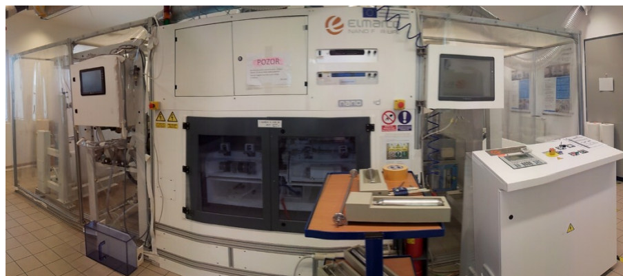
Figure 6:39 NanoSpider NS 4S1000U by Elmarco
