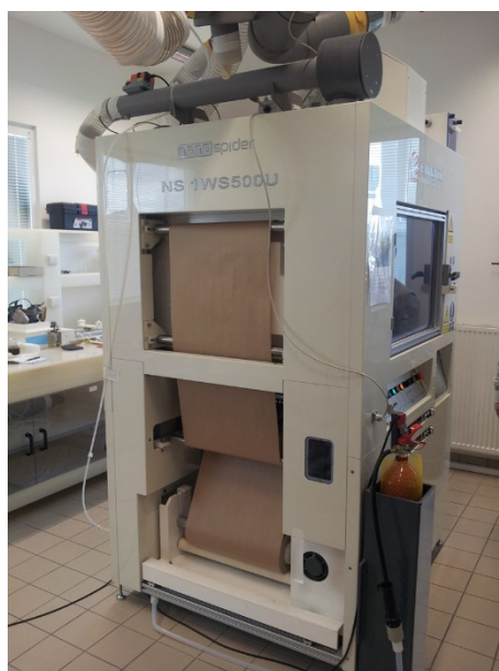
Figure 6:37 NanoSpider NS 1WS500U by Elmarco
