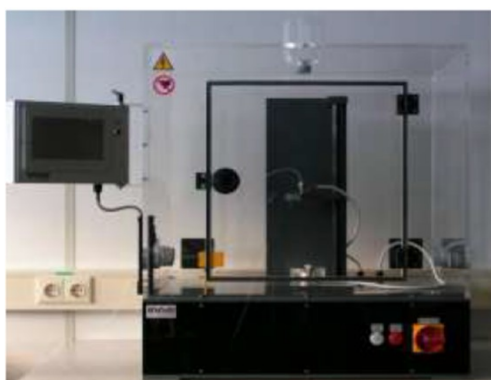
Figure 6:7 Electrospinning apparatus by IME Technology
