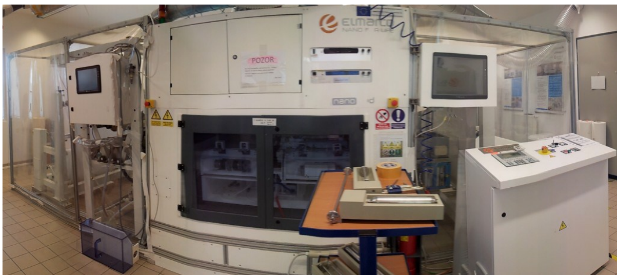
Figure 7.27 NanoSpider NS 4S1000U by Elmarco
