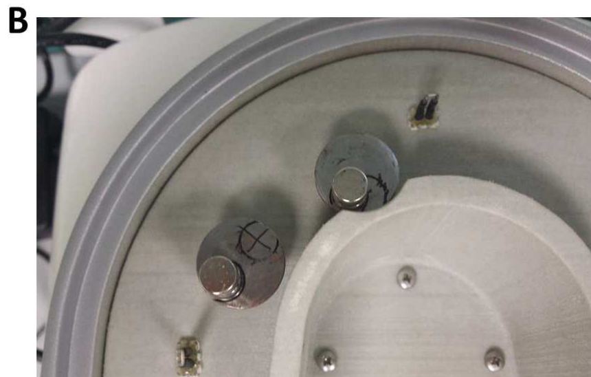
Fig.5. Magnets position: A) Qiagen disk player; B) P1B disk player.
