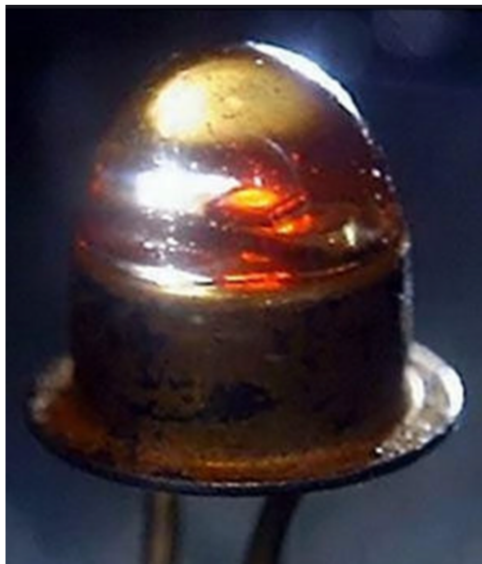
Figure 9.9: First GaAsP LED made by Holonyak
