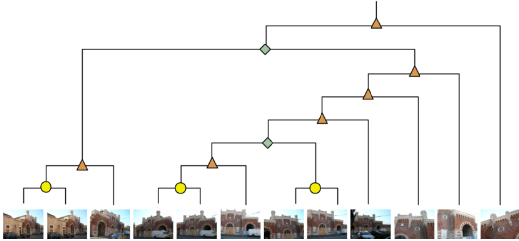
Figure 3.6: Example of hierarchical cluster tree in which on each internal node is associated the relative reconstruction operation. The circle corresponds to the creation of a stereo-model, the triangle corresponds to a resection-intersection, the diamond corresponds to a fusion of two partial independent models. 5
