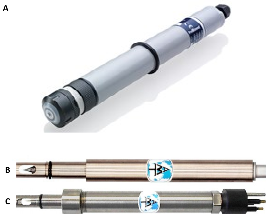
FIGURE 3.1 A) DULCOTEST \text{H}_2\text{O}_2 SENSOR; B,C) ATM PROTOTYPE
