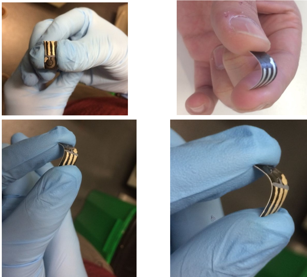
FIGURE 5.3 PICTURES SHOWING THE FLEXIBILITY OF THE PAPER BASED LASER SCRIBED DEVICE
