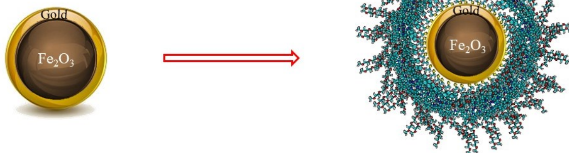
Figure 3.7.10: Synthesis scheme of the functionalization of Fe_2O_3@Au with porphyrins derivatives.
