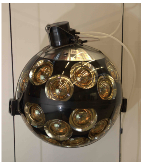
Figure 3.14: The DOM fixation on the two parallel DU-Dyneema ropes [7].
