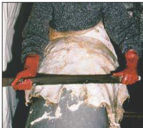
Fig. 19: After liming, the hairs and fat layers are removed with a blunt blade from the skin draped over a beam.
