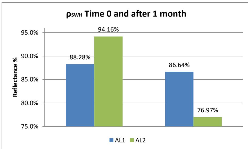
Figure 5. 132 Comparison between the solar weighted hemispherical reflectance for AL1 and AL2 sample in the "before" and "after" condition
