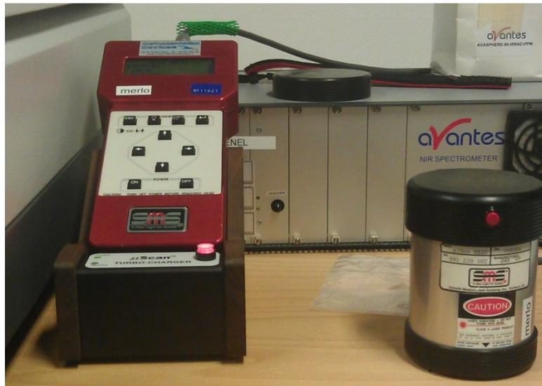
Figure 5. 88 SMS Scatterometer
