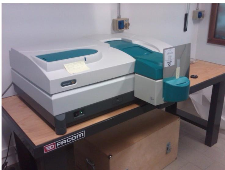
Figure 4. 1 Spectrophotometer Agilent Cary 5000
