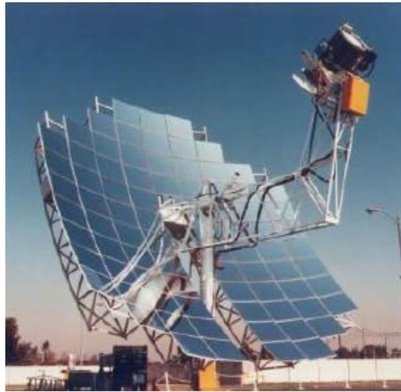
**Figure 2. 3 SES Dish/Stirling system**
