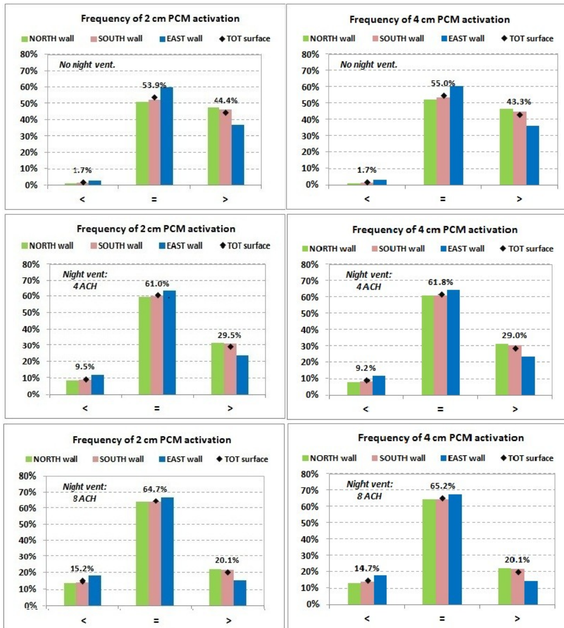
Fig. 42 Frequency of activation of 2 cm and 4 cm PCM panel.
